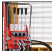
Distributore 4 leve Distributor with 4 levers
